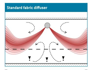
Warm air never reaches the occupied zone Because the duct is not optimised for only heating it must cool too.
